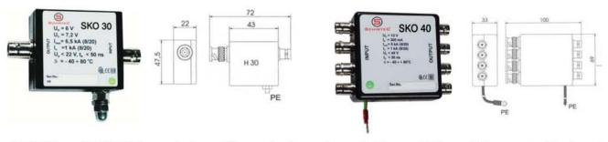
SKO 30 and SKO 30-L are designed for protection of coaxial lines of  $50\Omega$  or  $75\Omega$  against induced surge effects in the Lightning Protection Zones Concept at the boundaries of LPZ<sub>A(B)</sub>-1 and higher according to IEC 1312-1. They are used especially for protection of cameras and video signal concentrators. Applicable for security systems and fire control equipment.
